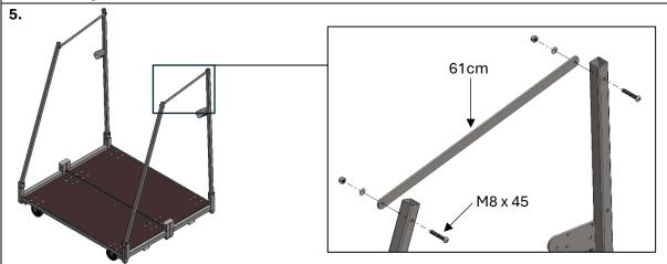
Do not overtighten the bolts. Posts must be able to move.
