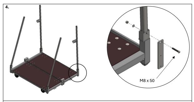
Do not overtighten the bolts. Posts must be able to move.
