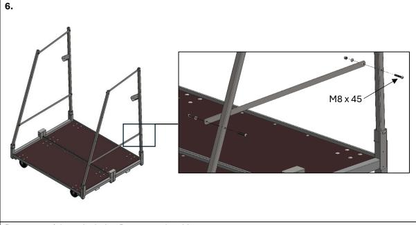
Do not overtighten the bolts. Posts must be able to move.
